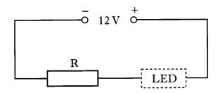
The voltage across the LED is 1.8 V and the current in the LED is 100 mA.
