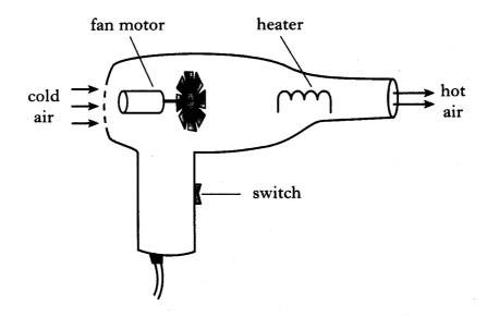
The heater and the motor both operate at mains voltage, 230 V.
