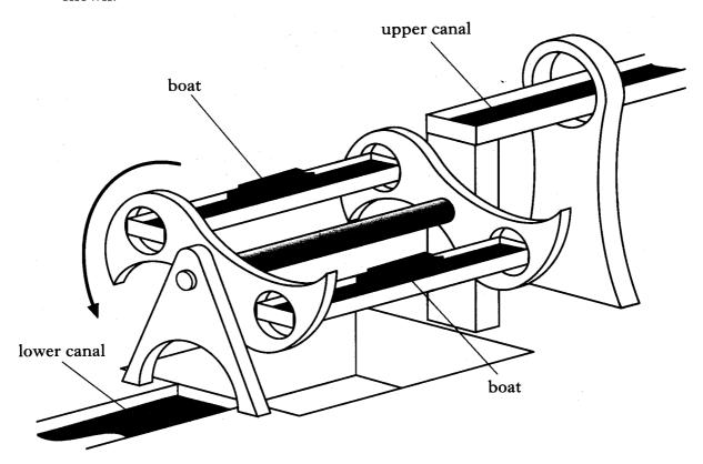
The lift rotates, lowering a boat on one side while raising a boat on the other side.
