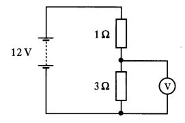
The reading on the voltmeter is
