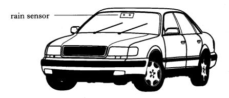
The rain sensor contains an LED which emits a beam of infrared radiation inside the car. In dry conditions this beam travels through the glass and is picked up by a detector as shown below.
