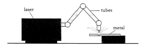
At one joint in the tube, the laser beam must change direction by 110°.
