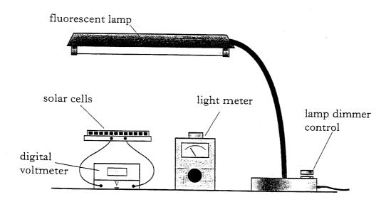
From her results, the student plots the following graph of the output voltage of the solar cells against the reading shown on the light meter.
