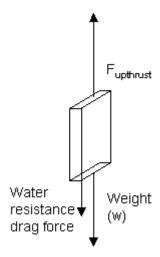
$$F_{un} = F_{upthrust} - (weight(w) + water resistance)$$
