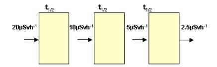
Three half value thicknesses are required. Thickness =  $3 \times 5 = 15mm$
