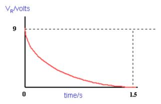
a.ii. The charging time is longer because less charge is transferred per second with a higher value resistor.
