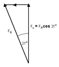
$$\begin{split} F_{\text{V}}(\text{total}) &= 2F_{\text{R}}\text{cos}21^{\circ} \\ F_{\text{V}}(\text{total}) &= 2 \text{ x } 4.5\text{x}10^{3}\text{cos}21^{\circ} \end{split}$$
