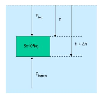
Only the difference in the depth( $\Delta h$ ) of the top and bottom surfaces affects the pressure difference.
