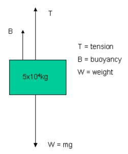
b.ii.Again as the manifold is stationary the upward forces balance the downward forces.
