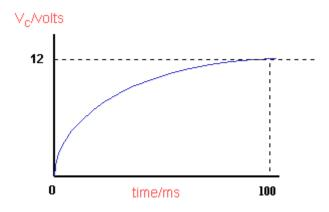
When fully charged the current in the circuit falls to zero and the voltage across the capacitor is equal to the supply voltage.
