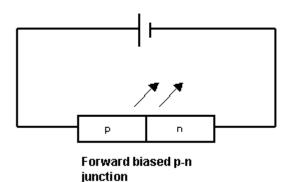
b. In forward bias the junction conducts if the applied voltage is high enough. Higher energy electrons flowing from the n-type material fall into holes, at a lower energy level, in the p-type material. The electrons give up energy in the form of photons as they do this.
