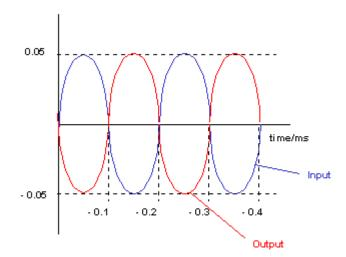
$$\begin{split} &V_{\text{output}}/V_{\text{input}} = -R_{\text{feedback}}/R_{\text{input}} \\ &V_{\text{output}} = -V_{\text{input}}x\left(R_{\text{feedback}}/R_{\text{input}}\right) \\ &V_{\text{output}}\left(\text{peak}\right) = -6x\left(3.0x10^3/2.0x10^3\right) \\ &V_{\text{output}}\left(\text{peak}\right) = -9V \end{split}$$
