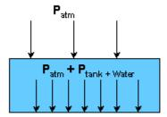
$P_{\text{total}} = P_{\text{tank+water}} + P_{\text{atmospheric}}$
