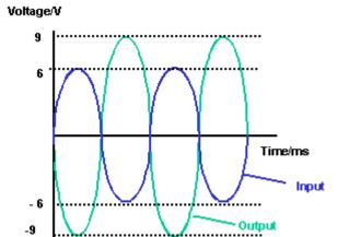
(B)  $V_{RMS} = V_{peak}/SQRT2$  $V_{RMS} = 9/1.414$  $V_{RMS} = 6.36V$
