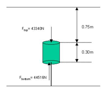
$F_{\text{upthrust}} = F_{\text{bottom}} - F_{\text{top}}$
