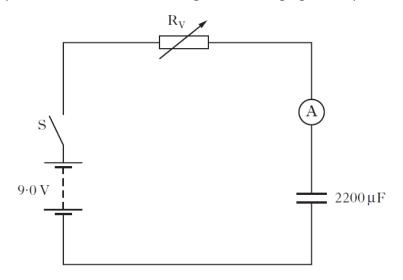
Initially the capacitor is uncharged and the variable resistor  $R_V$  is set to 12 k $\Omega$ .
