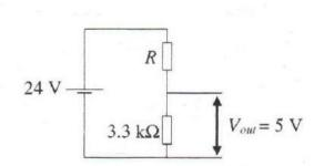
25. Find the output  $V_{\text{out}}$  from each of the following potential dividers :
