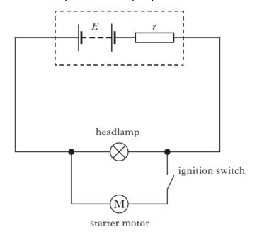
The technician notices that the headlamp becomes dimmer when the ignition switch is closed and the starter motor operates.
