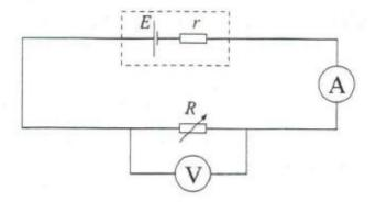
By varying the value of the load resistance R, the results in the table were obtained.
