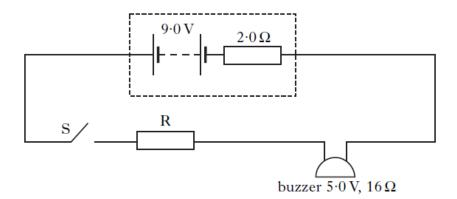
When the smoke is detected, switch S closes and the buzzer operates. The buzzer has a resistance of 16  $\Omega$  and an operating voltage of 5.0 V.
