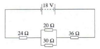
21. Find the reading on each meter in the circuit below.
