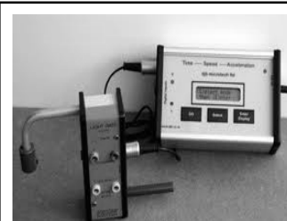
A light gate attached to a TSA meter. Apparatus you should be familiar with.
