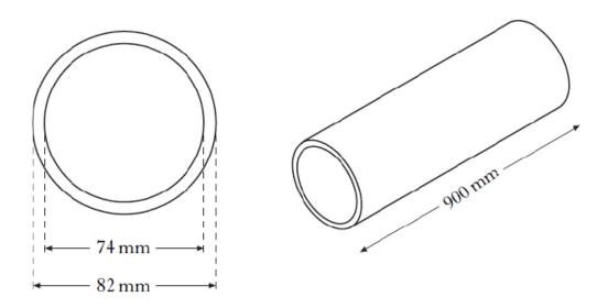
The inner diameter is 74 millimetres.
