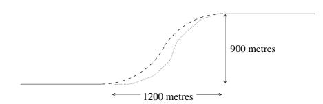
Two straight sections of a road, each running from east to west, and located as shown, are to be joined smoothly by a new roadway consisting of arcs of two circles of equal radius. The existing roads are to be tangents at the joins and the arcs themselves are to have a common tangent where they meet. 'Find the length of the radius of these arcs.
