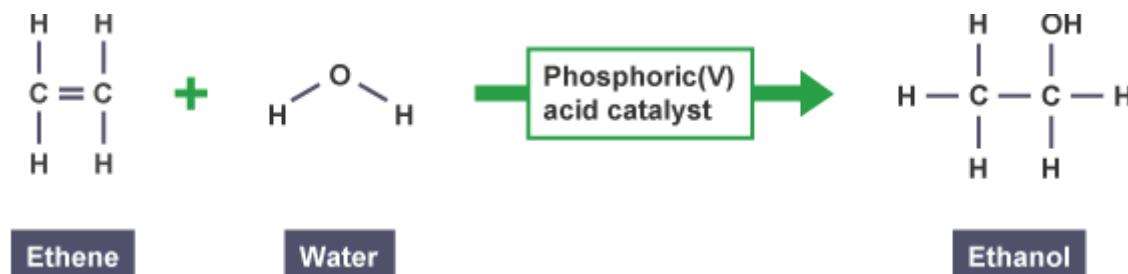
The addition of water to an alkene is called hydration and produces an alcohol.
