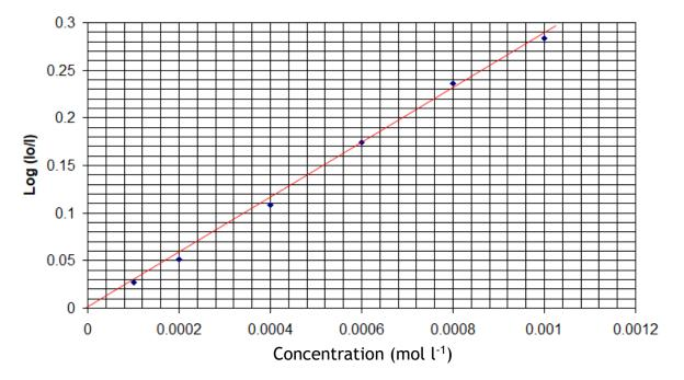
A sample of the  $Fe^{3+}$  solution was analysed in the colorimeter and found to have an absorbance of 0.15.
