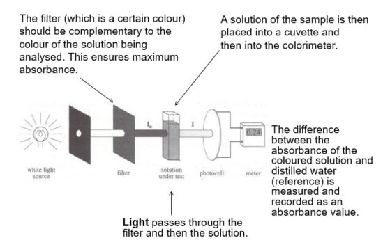
For any colorimetric analysis, it is important to prepare a calibration graph. This is achieved by carefully preparing several samples from a <u>standard solution</u> (solution of known concentration). This is done by <u>serial dilution</u>. The absorbance of each of these samples is measured by the colorimeter. It is important that a wide range of concentrations from the serial dilutions are obtained as this will ensure covering the concentration of the unknown sample.
