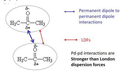
Pd-Pd interactions arise due to the permanent dipole caused by the difference in electronegativity between atoms in polar molecule.
