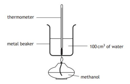
(C) The student burned 1.07g of methanol and recorded a temperature rise of 23°C.
