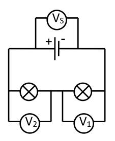
The voltmeter readings across the lamps in this circuit add up to the voltage across the battery.
