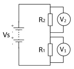
Drawn as above, the potential divider circuit is simply a series circuit following all the same rules; the current is the same at all points and the supply voltage splits up across each component to give them a share of the voltage (or potential difference).
