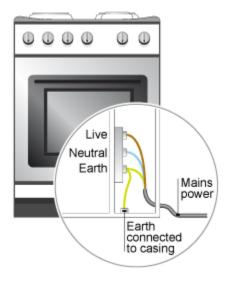
This can happen if the flex wiring becomes loose and touches the metal casing. Without the protection of the fuse and Earth wire the user would be electrocuted if they touched this live casing. The Earth wire is attached to the metal casing. If the metal casing becomes 'live' the high current drawn from the supply flows through the Earth wire (in preference the user touching the appliance) and at the same time the high current melts the fuse cutting of the power to the appliance.
