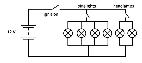
All the bulbs are placed in parallel with the battery so that each has 12 V across it.
