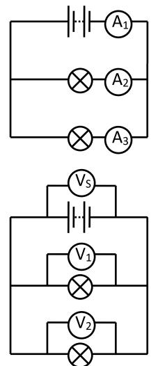
The currents through each component (branch) add up to the current from the battery.
