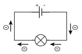
An **electric current** is the flow of electrons around a circuit. The greater the flow of electrons in a circuit, the greater is the current.
