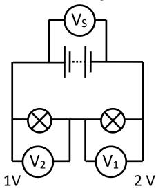
In a series circuit, the voltage across each component adds up to the supply voltage.
