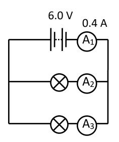
In a parallel circuit, the current from the battery is divided equally between the branches as the bulbs are identical.
