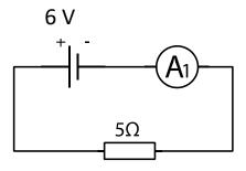
Calculate the value of current through the resistor.
