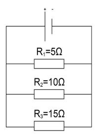
The **total resistance** of all three resistors in parallel is calculated using the following equation:
