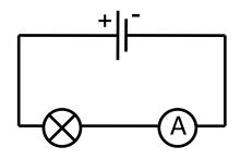
In the circuit, the ammeter is in series with the bulb. The reading on the ammeter is the current through the bulb.
