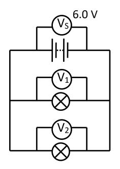
In a parallel circuit, the voltage across each of the components in parallel is the same as the supply voltage.
