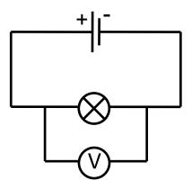
In the circuit, the voltmeter is added in parallel with the bulb. The reading on the voltmeter is the voltage across the bulb.
