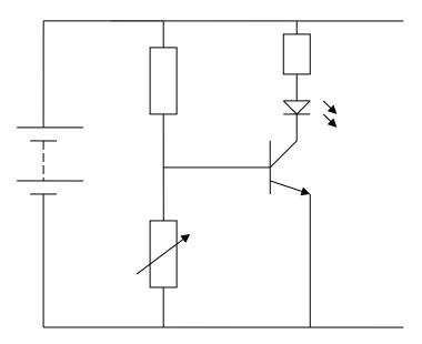
As the **resistance of the variable resistor is gradually increased**, the voltage across it increases and the voltage applied to the emitter-base increases. When the voltage applied to the emitter-base of the transistor is 0.7 V or more, the transistor will <u>switch on</u> and conduct allowing current to flow through it to the LED and the LED will switch 'on'.
