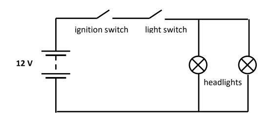
The two headlights are connected across the battery. They operate together only when the ignition switch and the light switch are on. The headlights are connected in parallel while the switches are connected in series.
