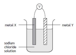
Which of the following pairs of metals would give the highest reading on the voltmeter?
