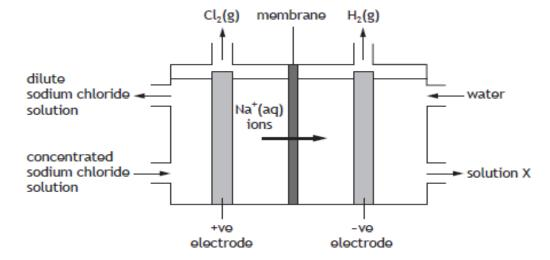
(a) Write the ion-electron equation for the change taking place at the positive electrode.
