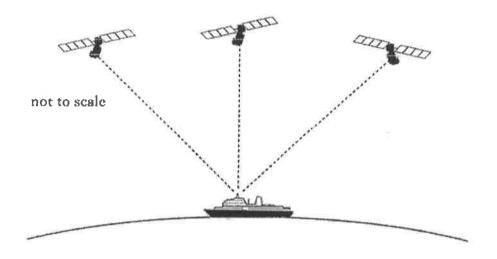
These satellites can transmit radio signals at three different frequencies, 1176MHz, 1228MHz and 1575MHz. The satellites orbit at a height of 20200km above the Earth's surface.
