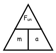
where:  $F_{un}$  is the unbalanced force acting on an object (N) m is the mass of an object (kg) a is the acceleration of an object (m/s<sup>2</sup>)
