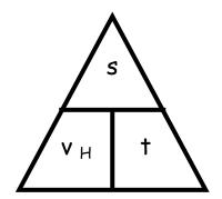
where:  $v_H$  is the horizontal velocity of an object (m/s) s is the horizontal displacement of an object (m) t is time taken (s)
