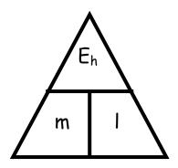
where: E<sub>h</sub> is the heat energy absorbed or given out by an object (J) m is the mass of a material (kg)
