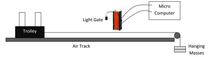
The acceleration of the trolley is measured. The value of the hanging masses is then changed thus altering the force pulling the trolley. The results of the experiment are shown.
