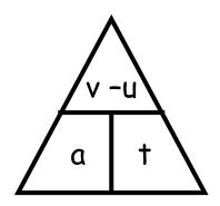
where: a is the vertical acceleration of an object  $(m/s^2)$   $v_v$  is the final vertical velocity of an object (m/s)u is the initial vertical velocity of an object (m/s)t is the time that an object accelerates for (s)
