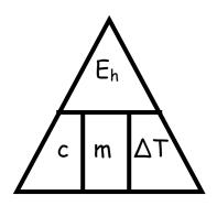
where:  $E_h$  is the heat energy absorbed by a material (J) c is the specific heat capacity of a material (J / kg °C) m is the mass of a material (kg)  $\Delta T$  is the change in temperature of a material (°C)
