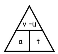
where: a is the acceleration of an object (m/s²)
