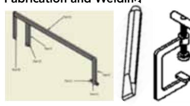
Using appropriate tools and equipment, including the forge and mig welder you will manufacture some items to demonstrate these skills, possibly the Hacksaw frame, cold chisel and G clamp shown above.
