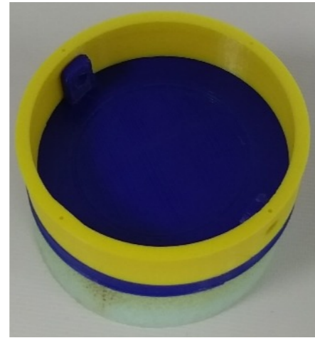
Line up holes on the insert and Middle housing
