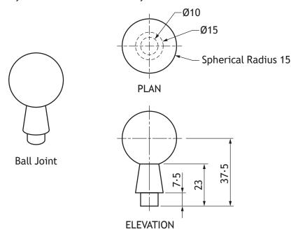
In order for the ball joint to work effectively a functional tolerance needs to be applied to it.
