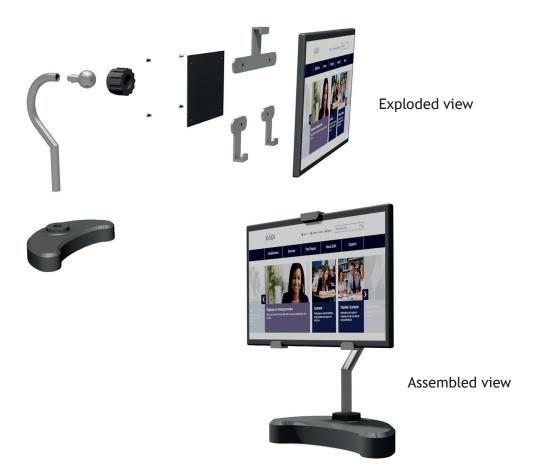
The tablet stand was designed using bottom up modelling.
