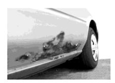
When painted on, rust remover changes iron(III) oxide into iron(III) phosphate.
