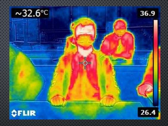
National 5 Physicists have been investigating the Electromagnetic Spectrum by using an infrared camera.
