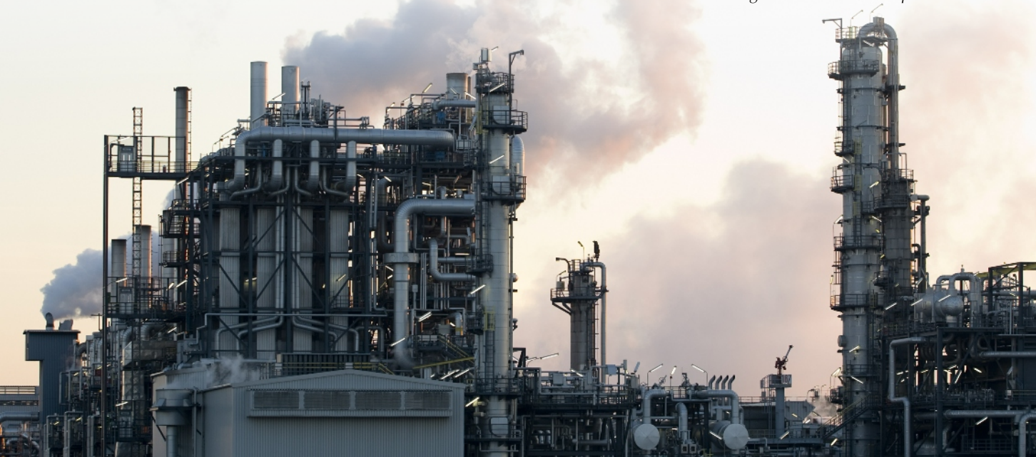
Petrochemicals require huge refineries to convert the complex hydrocarbons of oil into useful products used for making diesel, petrol and plastics. These plants have a large environmental impact.
