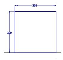
2. Finish the sketch and create a work plane. Offset the work plane 800mm.
