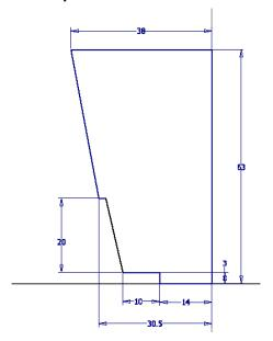
2. Use the revolve tool to revolve the profile 360° around the centre line.
