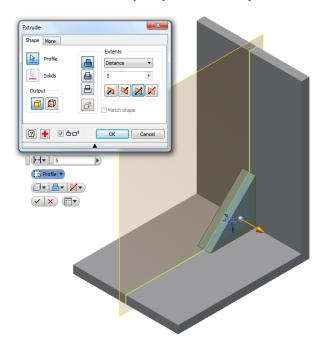
6. Create a new sketch on the upright surface and draw a 4mm circle as shown. Use the dimension tool to position it as shown.
