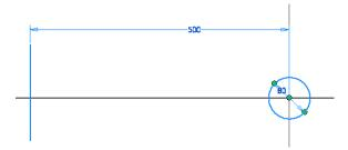
2. Select the revolve tool. Select the circle as the profile and the line as the axis and revolve 180°.
