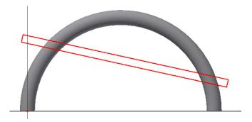
**5.** Finish the sketch and extrude the profile by subtraction into the arm of the chair by a suitable amount.
