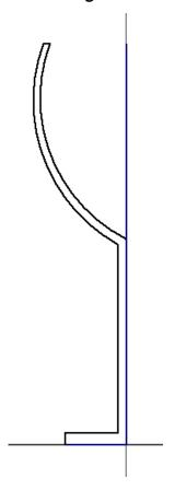
2. Use the revolve tool and revolve the sketch 360° around the centre line.
