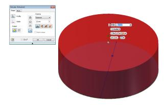
3. On the top surface of the cylinder, sketch a circle diameter 16mm.
