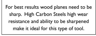
High Carbon Steel is harder but more brittle than lower carbon steels. It is still popular with many bush crafters and survivalists due to its toughness and ease of sharpening.
