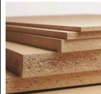
Chipboard is used when appearance and strength are less important than cost.
