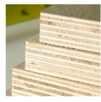
Plywood can be made up of a number of layers resulting in a variety of thicknesses. There is always an odd number of layers.
