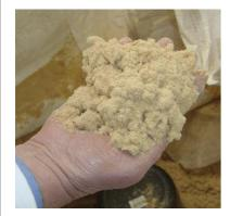
MDF boards are produced by tiny particles of timber glued together and then compressed with a resin adhesive.
