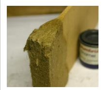
MDF can be easily damaged by moisture.
