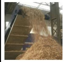
Chipboard is manufactured by mixing wood particles or flakes together with a resin and forming the mixture into a large sheet.
