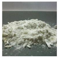
Cellulose Acetate is produced using wood pulp, which means less oil is used, making it a more sustainable material.
