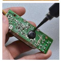
Epoxy Resin is a good electrical insulator.
