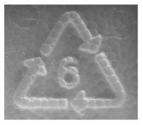
Expanded Polystyrene can be recycled and is represented by a number 6 in the recycling symbol.
