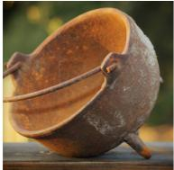
Cast Iron can have poor corrosion resistance.
