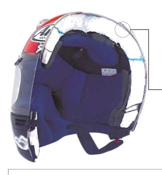
Inside the outer shell of a crash helmet is the impact absorbing liner, usually made of expanded polystyrene. The function of this layer is to absorb impact. The polystyrene compresses absorbing much of the impact. This system is designed to work one time. That's why a motorcycle helmet should be thrown away after being involved in a significant blow.
