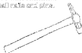
Cross Beak Hammer For small nails and pins.
