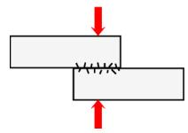
The glue soaks into the pores of the wood and then sets like lots of little fingers grabbing onto the wood on both sides. Using a cramp to hold the two halves of a joint together firmly helps to force glue into the pores of the wood. Cramping also holds the joint still while the glue is setting.
