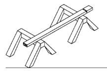
When sawing long pieces of wood, use a pair of **trestles** (also known as sawing horses). The wood can be held by G-clamps.
