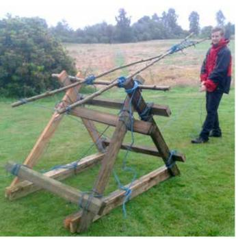
To fire the catapult place a soft projectile such as a soft toy or ball in the end of the arm A. Ensure that everyone is at least arms distance away from the catapult and that no one is standing in front of it. Pull rope B as hard as possible. Arm A will swing upwards until it is stopped by block C at which point the projectile will fly out.
