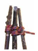
Pass both ends of the rope around each of the poles in turn going over one, under one, over one etc.
