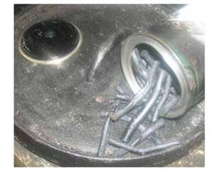
Charcoal is an impure form of carbon created by heating wood in the absence of oxygen so that the water in the wood evaporates. The carbon is unable to burn without oxygen so you are left with sticks of carbon.
