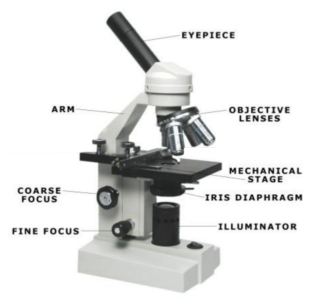
Stage to place the microscope slide on.
