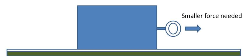
A lubricant is a slippery surface in a layer *between* the two surfaces. This reduces how much they rub together, so lubricants reduce friction. If there is less friction, there will also be less heat generated.
