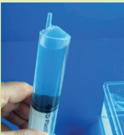
Figure 2b - Expel the air from the syringe before re-attaching.
