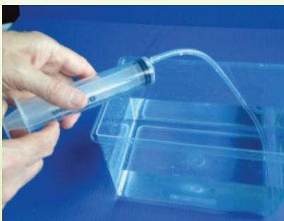
Figure 2a - Keep the end of the tubing under the water while filling the system.
