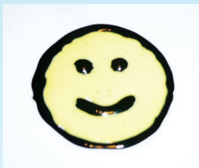
Figure 6 - Pick around the edge of the sticker and gently pull it off the acetate sheet. Place it on a warm surface and watch it change colour.
